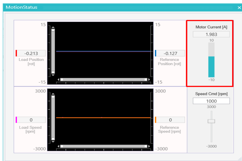
Figure 5. Monitoring the Motor current using the “Motion_Status” panel
