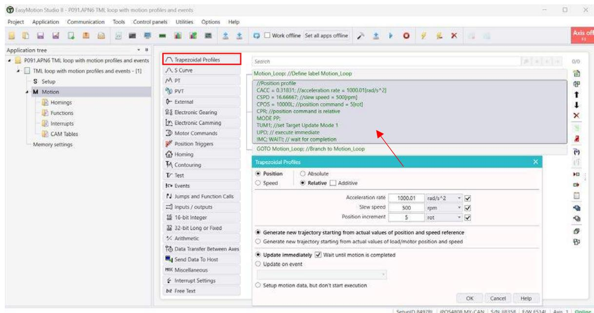
Figure 4 – Inserting a trapezoidal position profile
