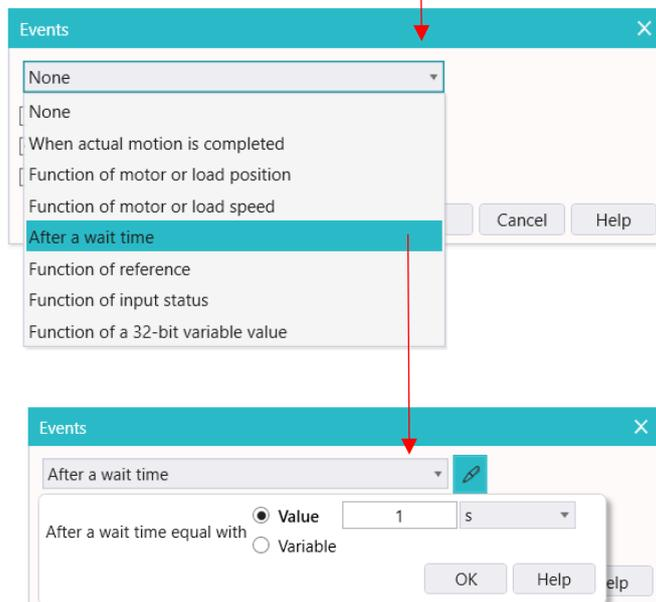
Figure 5 – Inserting a time event
