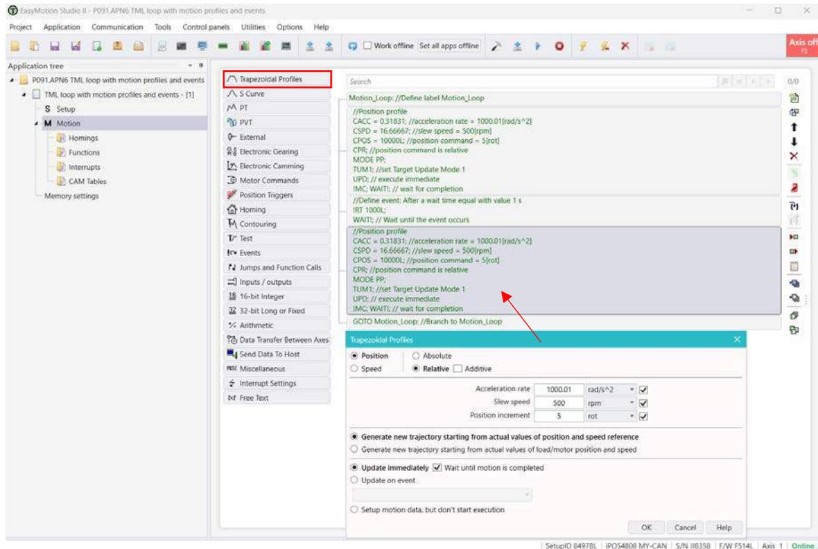
Figure 6 – Inserting a trapezoidal position profile
