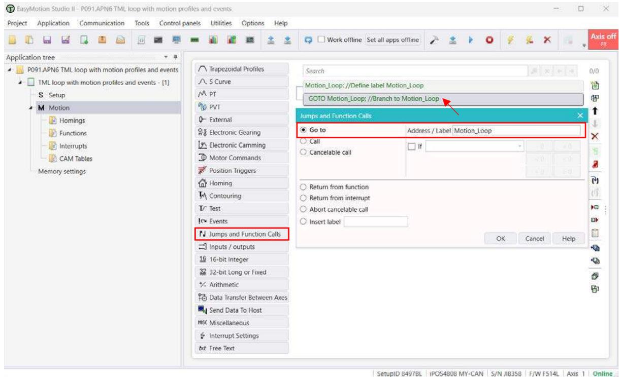
Figure 3 – Jump to Motion\_Loop label
