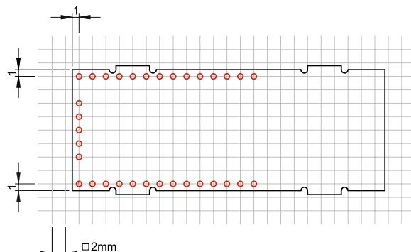
Top view; Pins facing downward; All dimensions are in mm; Header pitch is 2 mm.; Drawing not to scale; Tolerance  $\pm 0.1$ mm (unless otherwise noted)
