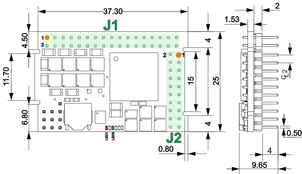
All dimensions are in mm. Drawing not to scale. Pins facing downward view.
