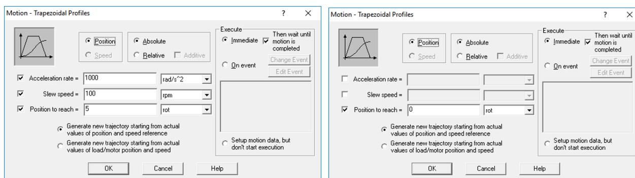
**Figure 7.** How to configure and start motion using a trapezoidal position profile
