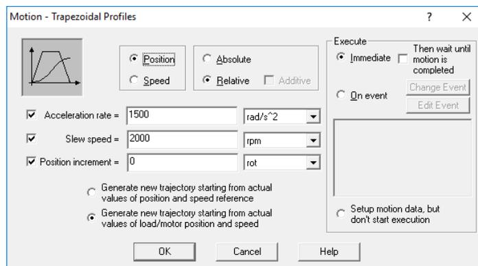
Figure 13. How to configure and start motion using a position profile using TUM0
