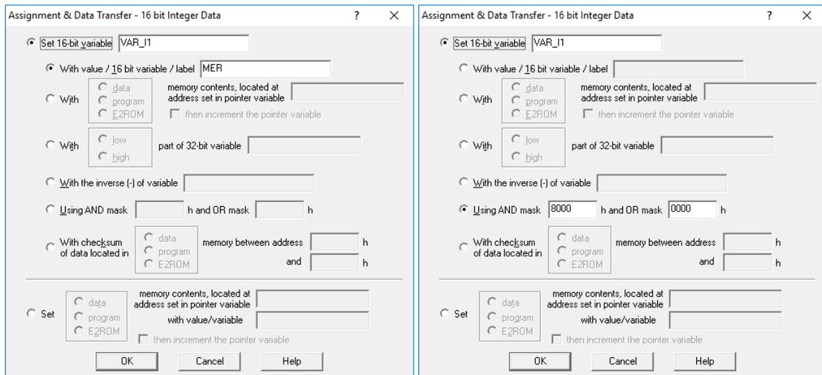
Figure 9. Operations using the “Assignment and Data Transfer – 16 bit Integer Data” dialog
