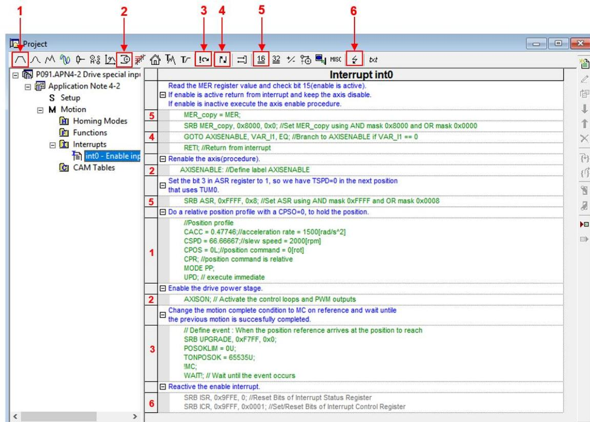
Figure 3. Enable Interrupt routine structure
