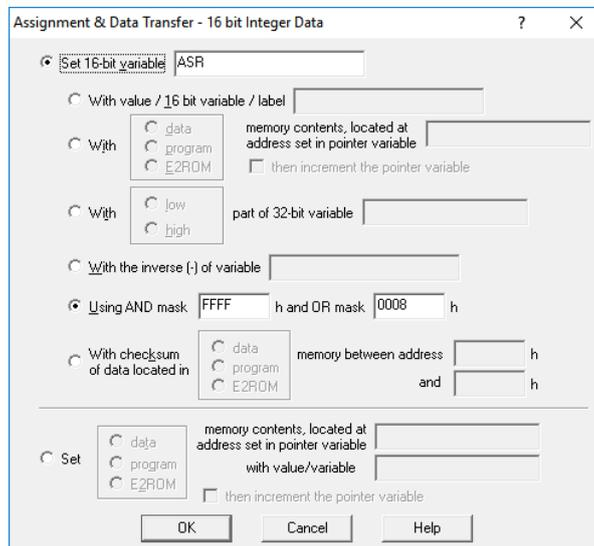
Figure 12. Set the bit 3 in the ASR register to 1
