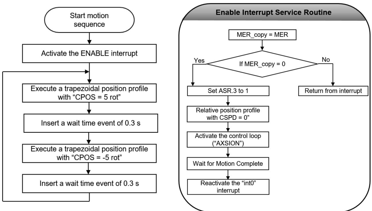
Figure 1. Enable TML interrupt structure & main motion structure
